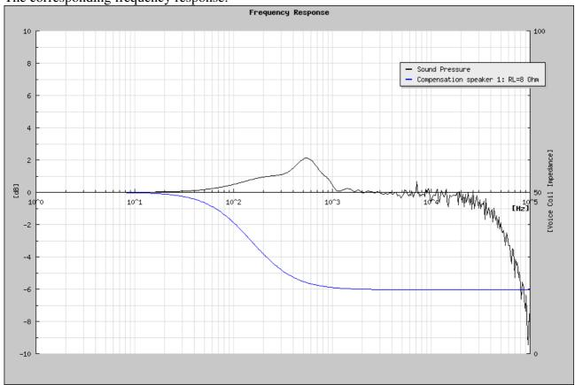
You can use the R2, C1, L2-network to attenuate another frequency: (R2=15Ohm, C1=100uF, L2=3mH)
